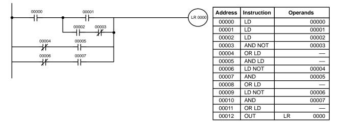
Although the program will execute as written, this diagram could be drawn as shown below to eliminate the need for the first OR LOAD and the AND LOAD, simplifying the program and saving memory space.
